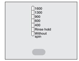
Press the "Spin" button repeatedly until the indicator light for the spin speed you want comes on.
